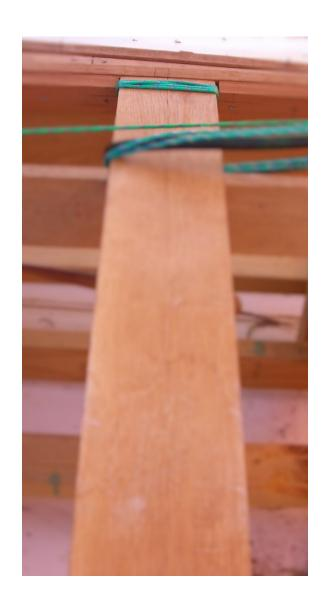
Keelson has been cut and let into the frame attached to the transom
