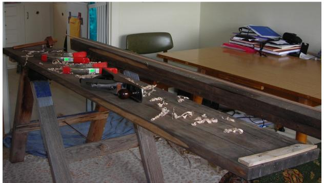
The tools are for working wood; I was able to access a supply of timber locally that provided me with a piece that I was able to cut down to stem size. A local man with a band saw trimmed to the pattern that I had drawn on the timber; some work with the spokeshave and: my stem!
