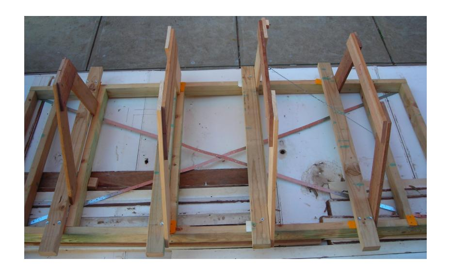
The moulds were cut out to allow the keelson to be set into the moulds.
