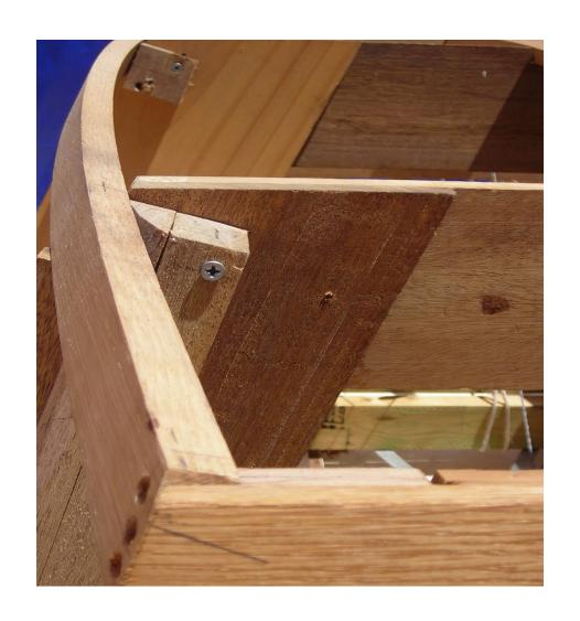
Now that the skeleton was in place it was time for the skin (planking) to be attached. Greg Rossel *Building Small Boats* was consulted and the idea of Lapstrake clamps led to the construction of this collection using the oak from the rejected chine.
