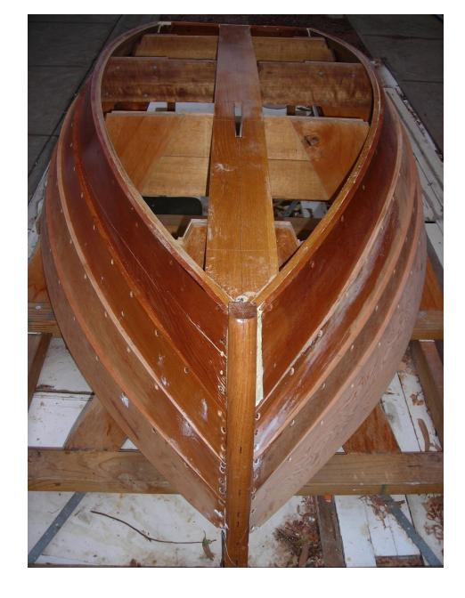
Eventually all the planks were in place and although they were not symmetrical (my need for balance was severely tested with this reality) the hull was in place.
