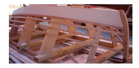
To make sure I had this process correct I created a model plank from 3mm particle board.
